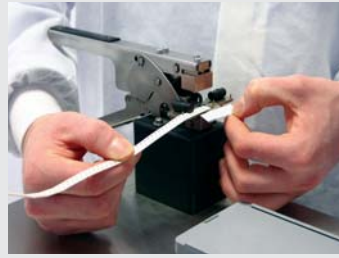
STEP 2 Place new component reel on splice clip
