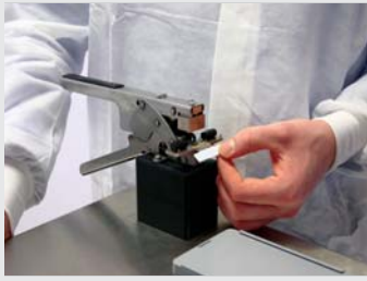
STEP 1 Put SMT Splice Clip into Tape Splicing Tool
