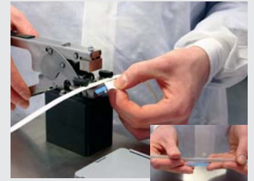
STEP 4 Remove backing paper from splice tape and join cover tapes with splice tape
